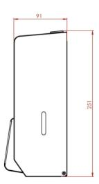
Height: 251mm Width: 108mm Depth: 91mm Weight: 1.2Kg Capacity: 900ml
