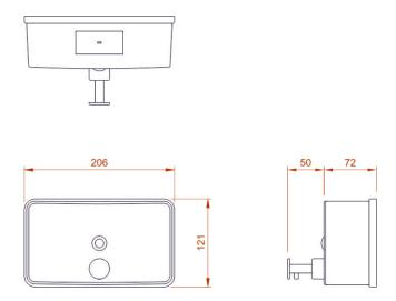
Height: 121mm Width: 206mm Depth: 122mm Weight: 0.6Kg Capacity: 1200ml
