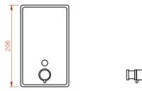
Height: 206mm Width: 121mm Depth: 122mm Weight: 0.6Kg Capacity: 1200ml
