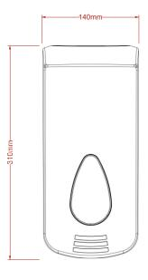
Height: 310mm Width: 140mm Depth: 145mm Capacity: 2Ltr
