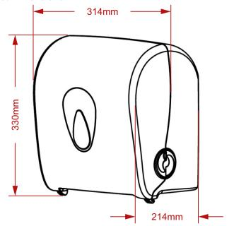
Height: 330mm Width: 314mm Depth: 214mm
