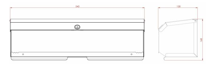
Height: 168mm Width: 540mm Depth: 158mm Weight: 2Kg Capacity: x1 20" Couch Roll
