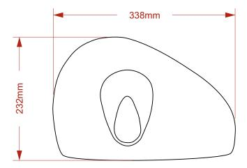
Height: 232mm Width: 338mm Depth: 123mm Capacity: 200mm Diameter Roll 100mm Diameter Stub
