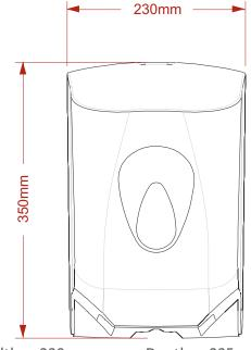
Height: 350mm Width: 230mm Depth: 235mm Capacity: 205mm Diameter Roll
