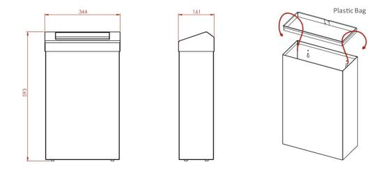
Height: 593mm Width: 344mm Depth: 161mm Weight: 6Kg Capacity: 30 Litre
