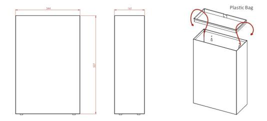
Height: 527mm Width: 344mm Depth: 161mm Weight: 4Kg Capacity: 30 Litre
