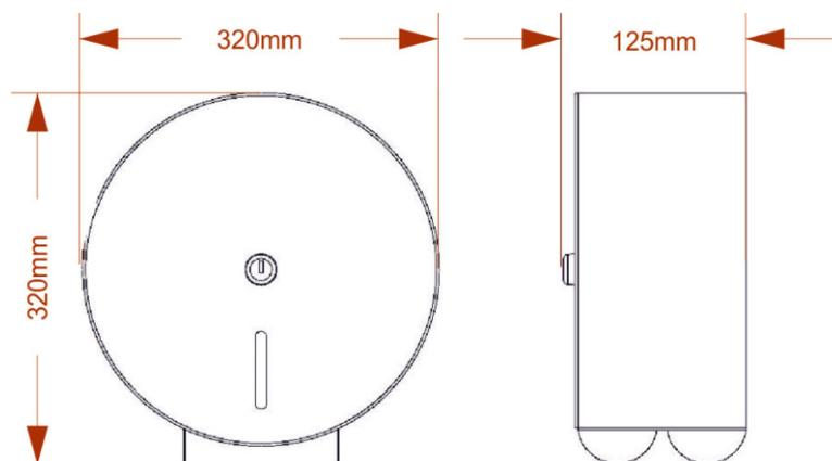
Height: 320mm Width: 320mm Depth: 125mm Weight: 2Kg Capacity: 320mm Roll
