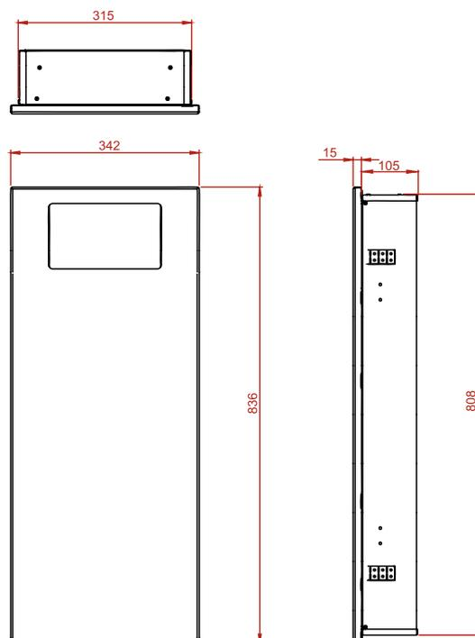
Height: 836mm Width: 342mm Depth: 120mm Weight: 9Kg Capacity: 18 Litres
