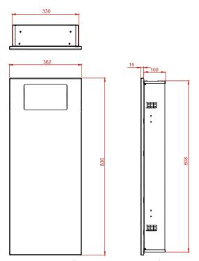
Height: 836mm Width: 362mm Depth: 115mm Weight: 9Kg Capacity: 18 Litres
