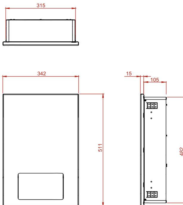
Height: 511mm Width: 342mm Depth: 120mm Weight: 6.4Kg Capacity: 400/500 Towels
