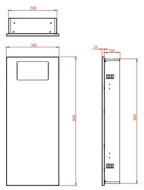
Height: 836mm Width: 342mm Depth: 115mm Weight: 9Kg Capacity: 18 Litres
