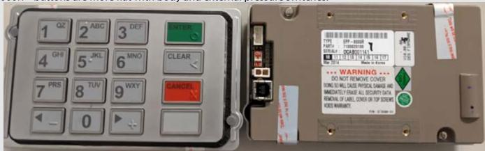
EPP-X1 – Additional paneling that prevents easy access to back of keypad, external pressure switches.
