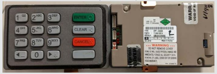
8000R – buttons are more flat with body and external pressure switches.
