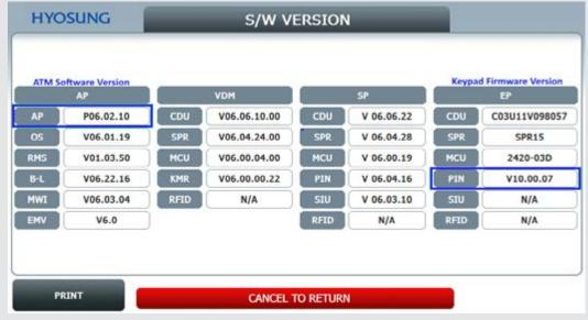
EP PIN Versions of 10.0x.xx or higher are compatible with TRI-31 PCI requirements
