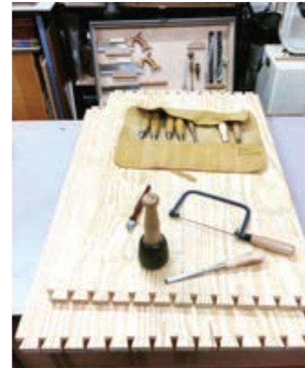
Cutting multiple dovetails is an ideal way to embed skills and display one's abilities
