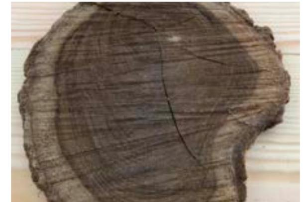
Part of the log delivery (left) deposited in the workshop foyer. Time for a cup of tea... Bill cut a 20mm slice from the end of one log and exposed the vivid colour difference between the oxidised (above) and freshly exposed timber (below)
