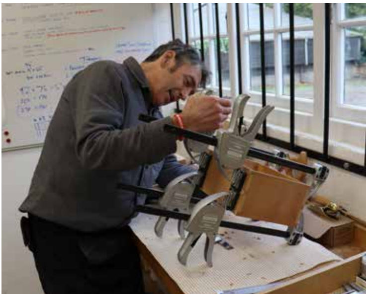
Fish glue was used for the assembly of a dovetailed box when Nick Gibbs (left) visited Bill's workshop last year. Using a syringe (above) to fix a loose piece of veneer
