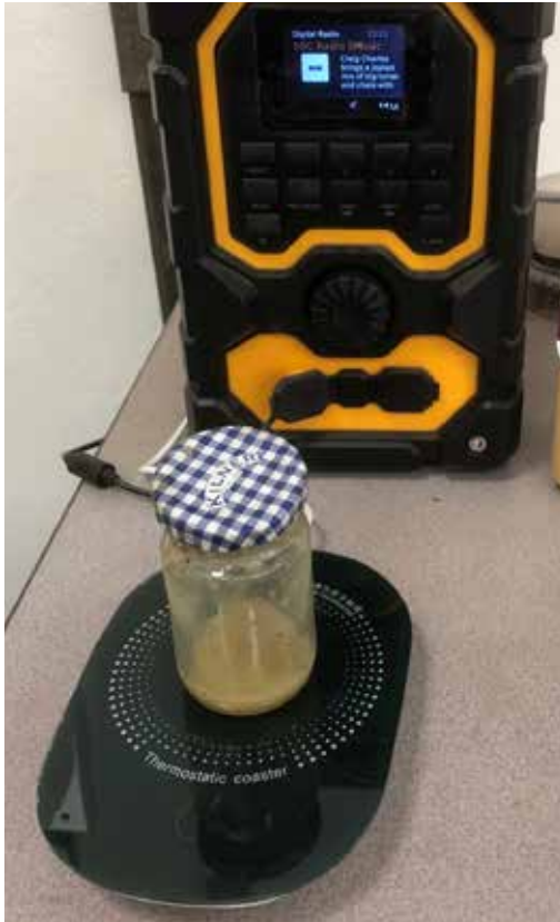
Bill also uses a ThermoTastic Drink Coaster (above), powered via USB from the back of a DAB radio. The weight of the bottle switches on the heat and is very gentle and hot enough to warm a pot of glue on even a cold day
