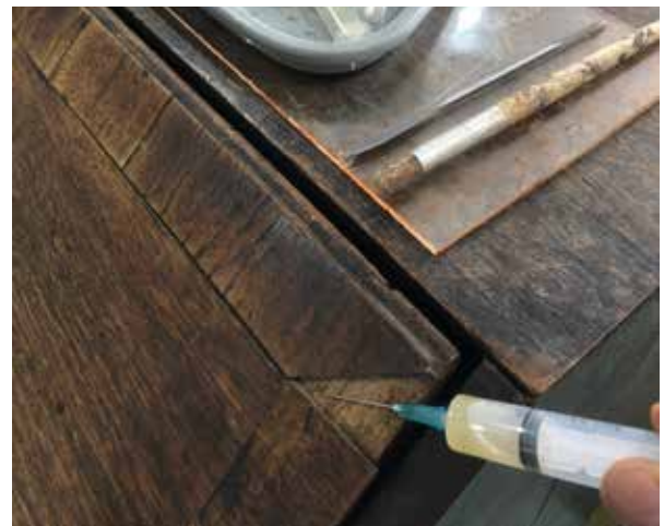
Fish glue was used for the assembly of a dovetailed box when Nick Gibbs (left) visited Bill's workshop last year. Using a syringe (above) to fix a loose piece of veneer
