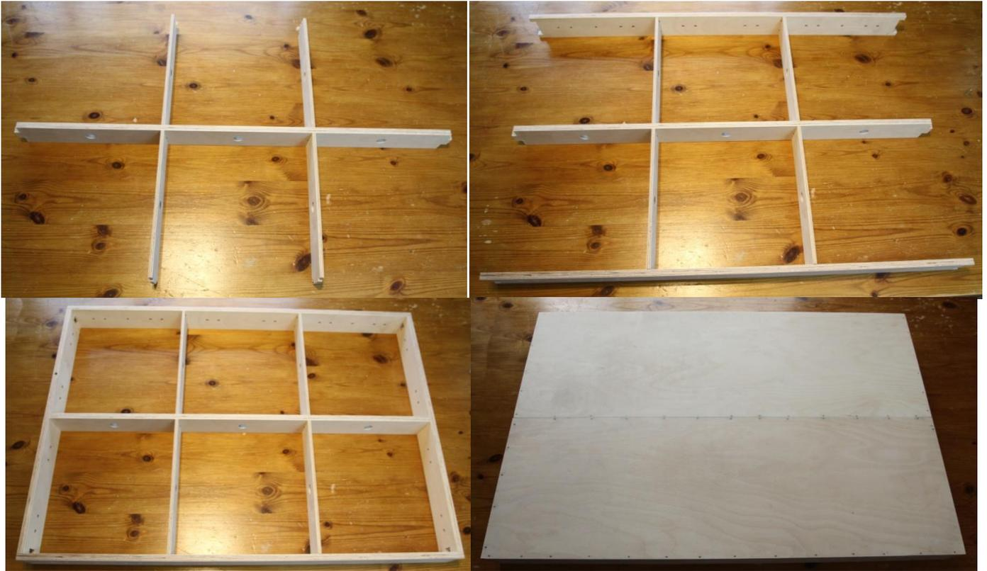
Assembly is similar to the narrower baseboards with the addition of two extra screws in each end as below:
