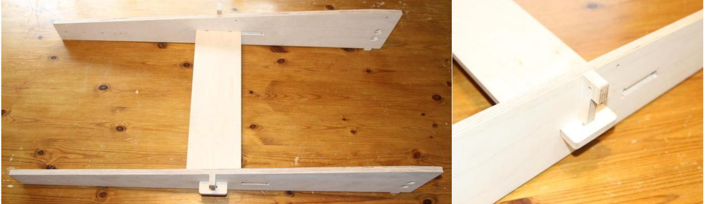
The leg assembly is fitted to the baseboard simply by slotting the locating pegs into the rectangular holes in the end and then fitting the bolts as below.
