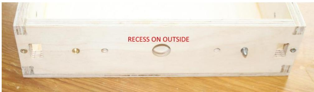
Offer this baseboard up to the other and locate the corresponding holes, these will not be the outermost ones if the other board is wider than this one.
