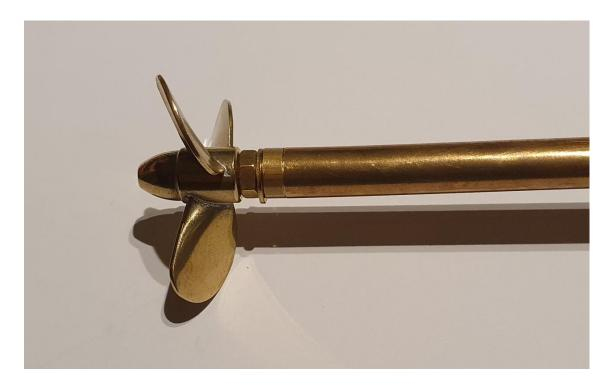
On the front there's a brass thrust collar with locking grub screw, then the coupling and motor (optionally included in the kit)
