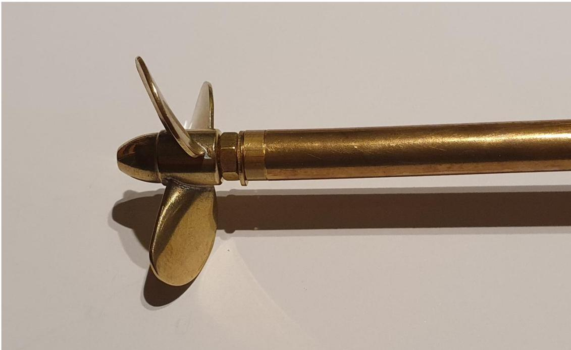
On the front there's a brass thrust collar with locking grub screw, then the coupling and motor (optionally included in the kit)
