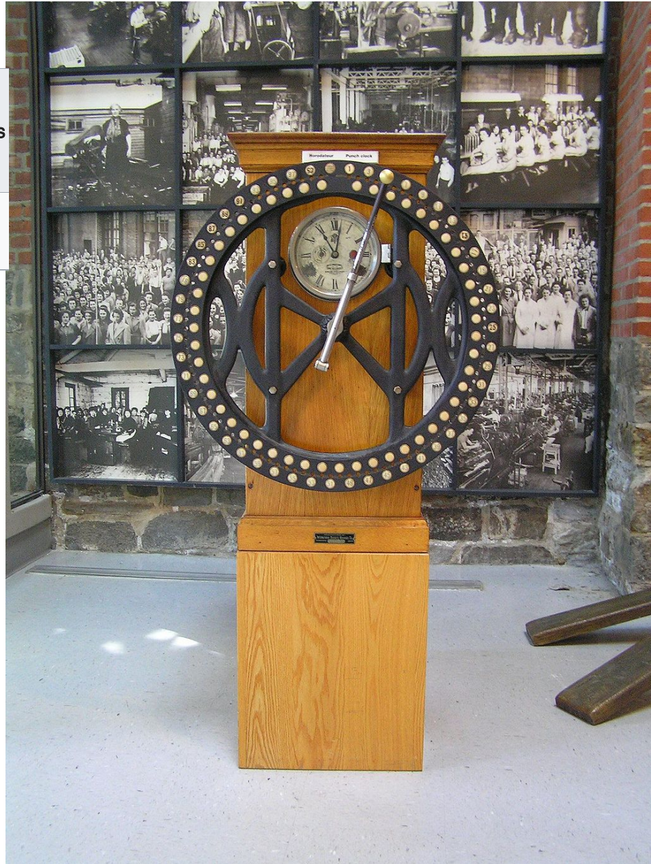
IBM International Daily Dial Attendance Recorder. 1930s time clock made by IBM's International Time Recording division. The face shows employee numbers which would be dialed up by employees entering and leaving the factory. The day and time of entry and exit was punched onto cards inside the box. [37]
