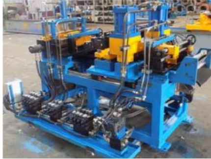
Auto Coil Joining Equipment
