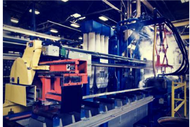
In-Line Induction Heater with Fume Extractor System
