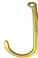
#N711-2 Forged 15" J Hook with eye 4 lbs WLL 5400 lbs
