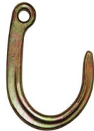
#N711-10 Forged 8" J Hook with eye 3 lbs WLL 5400 lbs
