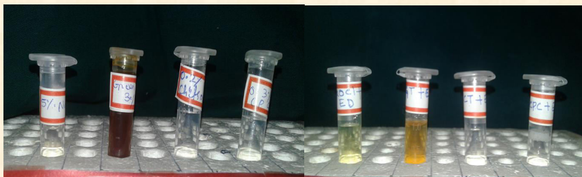
Figure 3: Grouping of the samples with and without addition of etidronic acid
