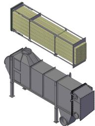
In the past, we have also for the flue gas coolers and heat exchangers used old-fashioned technology that reliably fulfilled its tasks, but reached its limits in the area of wear and tear and also in maintenance. In the same order as we did with the combustion grate system we took a closer look at these problems and created a new type of flue gas cooler that is very easy to maintain.
