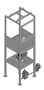
A dry-scrubbing-solvent injection by means of a dosing station is used to remove particles and gases from the exhaust gas streams via dusted air filters.
