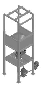
A dry-scrubbing-solvent injection by means of a dosing station is used to remove particles and gases from the exhaust gas streams via dusted air filters.
