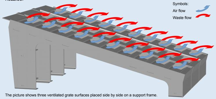
The air swirl with a huge amount into the combustible materials and convey them along the grate. The swirling combustion air turns over the combustible materials, cracks it up and assist the whole combustion process. Therfore also a high throughput rate is achieved per unit area of grate.
