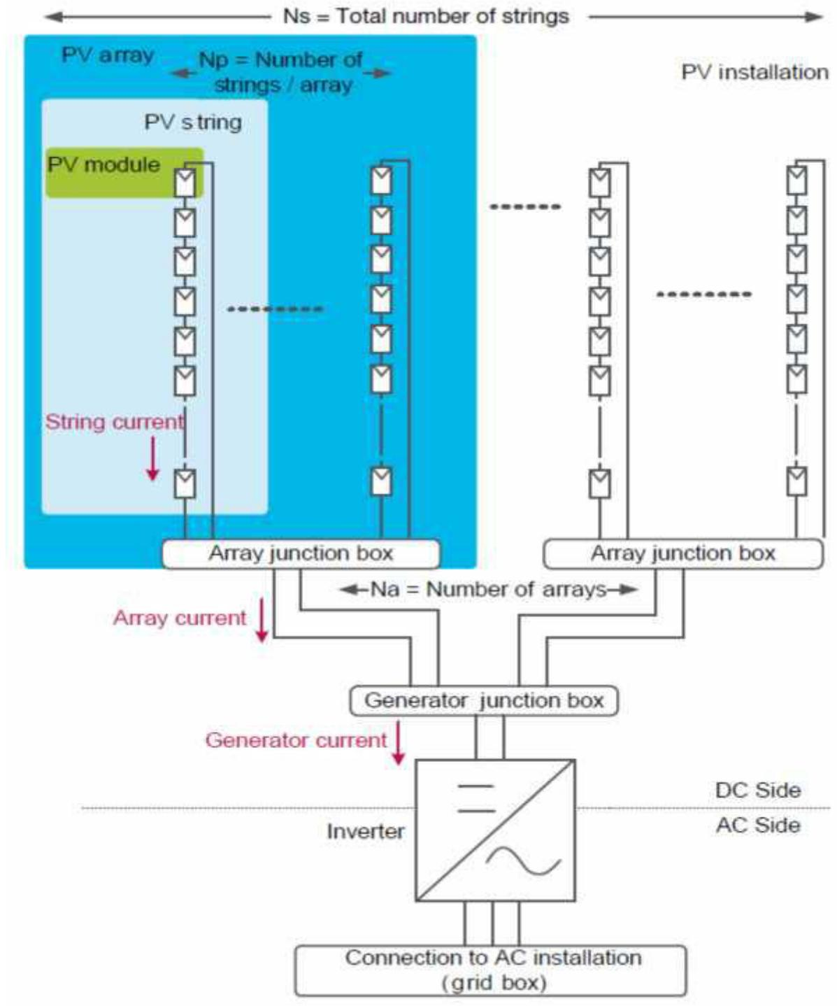
The diagram is made for 1MW block calculation
