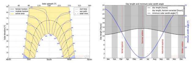
Left: Path of the Sun over a year. Terrain horizon (drawn by grey filling) and module horizon (blue filling) may have shading effect on solar radiation. Black dots show True Solar Time. Blue labels show Local Clock Time.
