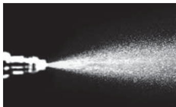
Injector spray pattern after P.i. treatment.
