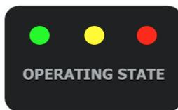
The operating state of the instrument is indicated by 3 colored light emitting diodes (LEDs). The green diode is on when the instrument is turned on. The yellow diode indicates that the WiFi antenna is ready to transmit and receive data. The red LED will in general blink when the instrument is busy with either measurements or analysis
