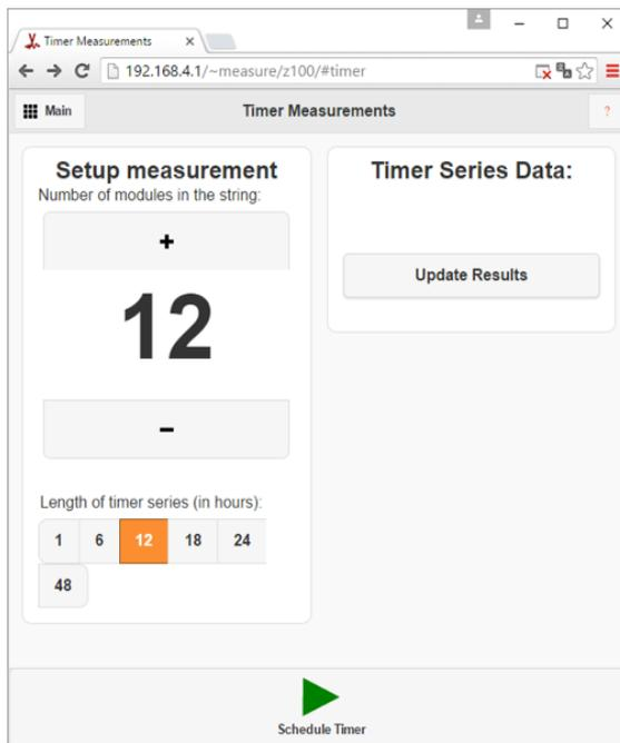
The number of PV modules "N" must be adjusted using the + and - buttons. Select the duration/length of the timer test using the buttons: a ground fault test will be conducted every 15 minutes during the duration of the test. The Schedule Timer button will start the test when pressed. The WiFi antenna will close down during test
