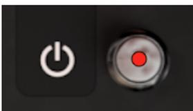
When the timer function is active the diode will change colour from bright green to red (WAKE UP state). If the button is pressed in the WAKE UP state, the timer test will be interrupted, and the instrument will wake up to normal operation.
