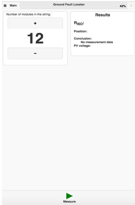
First enter the number of PV modules using the + and - keys. The measurement will take 45-60 seconds. In the **Results** window the measured  $R_{ISO}$  together with the string  $V_{OC}$  are returned. After the measurement is done, you can download a PDF report with the results to your device for documentation purposes. Simply press the **Generate report** button, and follow the instructions in the GUI.
