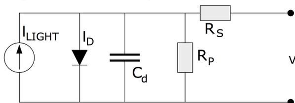
Solar module string - equivalent circuit. This model is roughly equivalent to the solar module string, and a basis for understanding the impedance measurement.
