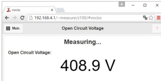
Voltage is shown instantly. In the example to the right almost 410V is measured across 12 x 250 W mc Silicon modules indicating irradiation close to Standard Test Conditions.
