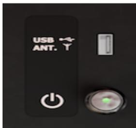
Placed on the middle of the front panel we find the ON/OFF switch. When the instrument is turned on a small LED in the button will emit green light. The ON/OFF button also controls the "Timer" application. This application is described in detail in the Timer section.
