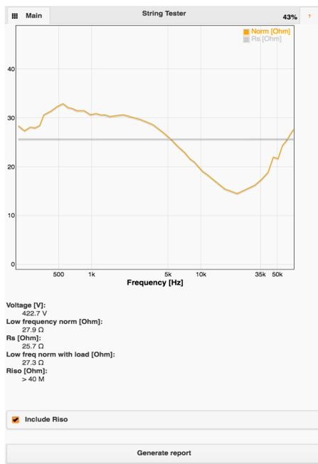
Connect the instrument to the PV string and press the **Measure** button to collect a spectrum. The measurement will take 30-60 seconds. In the example shown to the right,  $R_S$  is  $16.9 \Omega$  as is the low frequency norm at a voltage of close to 410V, which indicate a healthy string of 12 x 250 W modules with a decent sun irradiation. With a higher irradiation  $R_S$  could go as low as  $10 \Omega$ .
