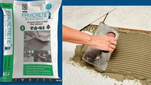
**Coverage:** Approx 55-60 sq. Ft. Per 20 kg bag with a  $\frac{1}{4}$  x  $\frac{1}{4}$  (6mmx6mm) square notch trowel for a bed of 3 mm (Consumption may vary depending on the evenness on the substrate, trowel notch size, type of tile and application technique)
