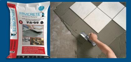
**Coverage :** Approx 55-60 sq. Ft. Per 20 kg bag with a ¼ x ¼ (6mmx6mm) square notch trowel for a bed of 3 mm (Consumption may vary depending on the evenness on the substrate, trowel notch size, type of tile and application technique)
