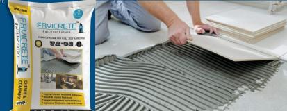
**Coverage :** Approx 55-60 sq. Ft. Per 20 kg bag with a  $\frac{1}{4}$  x  $\frac{1}{4}$  (6mmx6mm) square notch trowel for a bed of 3 mm (Consumption may vary depending on the evenness on the substrate, trowel notch size, type of tile and application technique)
