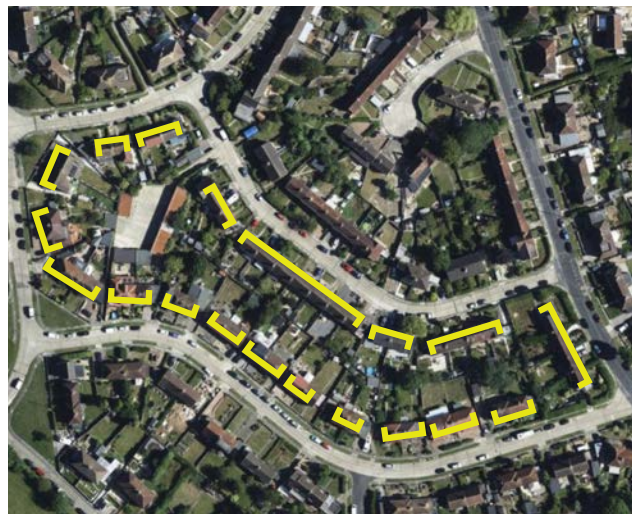
New development should follow a consistent building line and orientation as is observed from the immediate surrounding context to form a unified built environment.
