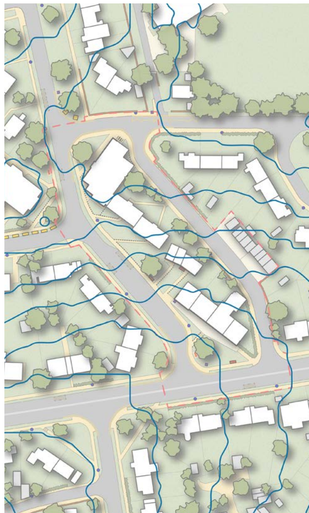
Figure 41: LIDAR 2m contour map within the Beatty Avenue village hub.
