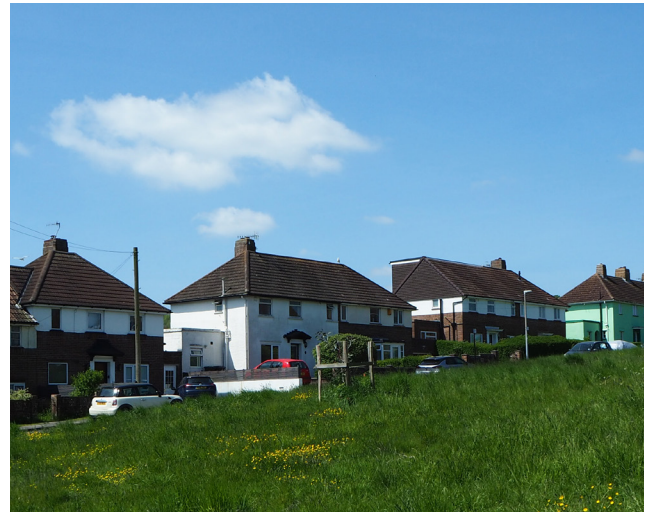
Street-facing roofline has a consistent angle, material and colour palette, chimney placement and rhythm. Flat roof dormers are set behind the building so as not to disrupt the uniform street scene.
