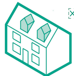
Inappropriate dormers which contrast existing fenestration.
