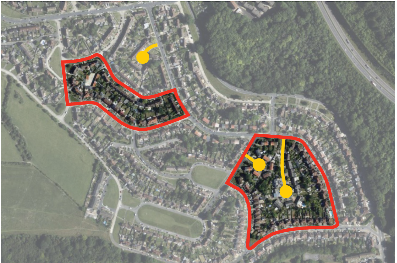
Example of a curvilinear residential block (upper perimeter - red), a short cul-de-sac development (upper line - yellow) and a mix of the two with multiple tandem infill cul-de-sac developments occurring within a large residential block (lower right).
