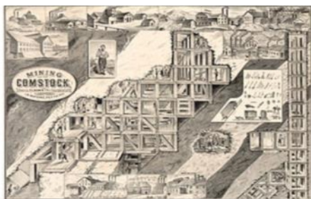
From Wikipedia, the free encyclopedia "Mining on the Comstock", depicting the headframes and mills of the various mines, and mining technology used at Comstock, most prominently the method of square-set timbering developed there to work the veins.
