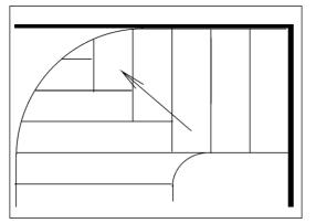
**C)** a slope - Corners - This method is used mostly for shorter slopes to cap waste landfills or for fractional slopes of oblong waste landfill shapes.
