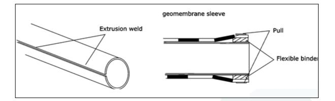
A pipe is fastened to the geomembrane sleeve by a pulling collar (the pull) and by sealing material. We recommend to use two pulling collars. D) Other was of joining pipes from other material than the geomembrane is made of is joining by means of a firm and a loose flange.
