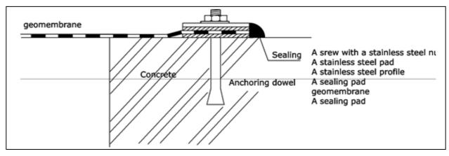
Distance of screws depends on a solidity of an anchoring ledge, or of an anchoring profile (for steel amchoring plate 10 mm thick the distance should not be bigger than 150 mm). It is also possible to anchor the MACLINE geomembrane to concrete by a HDPE anchoring element. This anchoring element is installed already during concreting itself and the MACLINE geomembrane is anchored to it by an extrusion weld.
