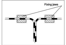
The peeling test is considered successful if a sealing sheet has been prolonged next to the weld (so-called a plastic deformation) and then the geomembrane sheet **has been torn outside the weld.**
