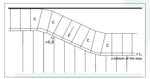
Ending of the geomembrane sheet laid on the slope must not be done at the bottom of the slope. A minimal distance from the bottom is 1,5 m. A minimal distance of two (T) joints from each other should be 0,5 m.
