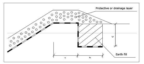
We recommend to use bench on long slopes. Sealing can here be fixed by terrestrial inter-ditch.
