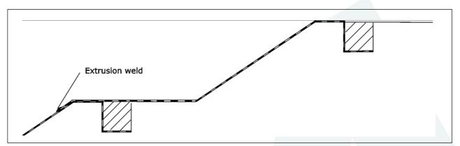
An important factor is to ensure a temporary stability of the geomembrane for the time when the anchoring ditch is not finished (properly earth-filled and firmed). The geomembrane can be partly pulled out from the notch because of temperatures influence and that way its influence on the geomembrane stability can be reduced. We recommend to anchor the geomembrane by steel hooks or by a similar way to the bottom part of the terrestrial ditch.
