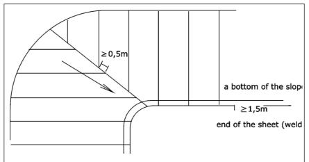
B2) a tree - overlapping - This method is mostly used for waste landill capping
