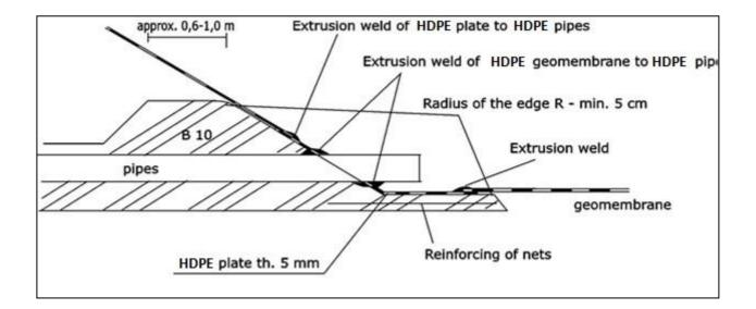
B) Pipe penetration through sealing with use of more sealing layers
