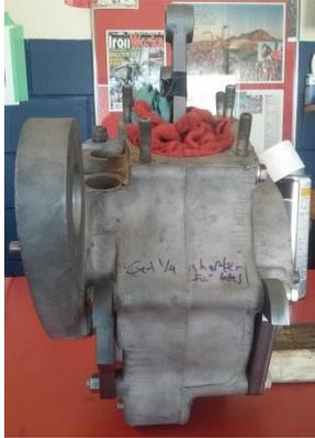
2. Mock up the front shelf across the two side brackets bolted to the case and clamp them together using square blocks.
