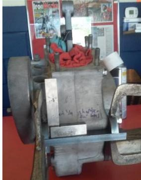
3. At this point, you will want to move on to the rear motor mounts and get them mocked up, the engine located to the lateral position needed, squared, and aligned with the belt drive to the transmission.
