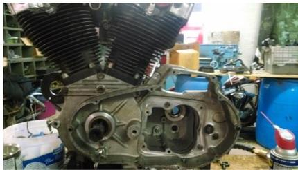
1. To begin this process remove the primary cover, primary, clutch basket, trap door transmission, starter assembly, cam cover, cams, and oil pump. Clean off the engine as best as you can and using brake clean prep the surface so you can mark where you are supposed to cut. Mark out as straight of a line as possible marking where to cut as shown.
