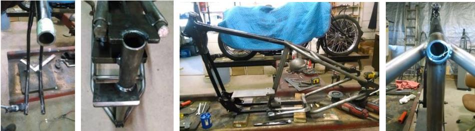
**79-81 FRAMES:** these three years of frames have an odd design. Most of this will get cut off. The only differences is the back bone. The area where it is to be plugged has been dented for factory clearance. You have two options. **1:** using a torch heat up the dented tube and pound out the dent allowing the plug to be inserted. **2:** cut out the dent and add an extension to replace the
