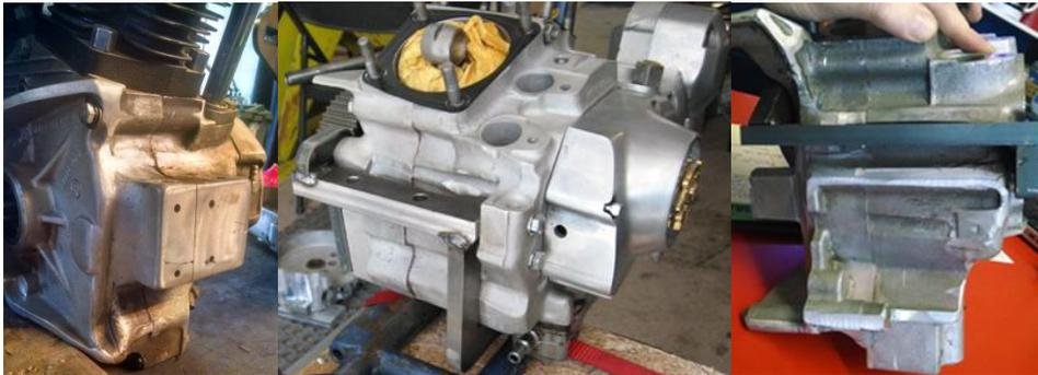
**FRONT:** The front motor mounts is NOT needed to build an original frame Shortsters conversion. The front motor mount set converts Sportster motor mounts to Big-twin style in height and longitudinal location for custom frame applications. The bar is undrilled for your desired lateral engine position.
