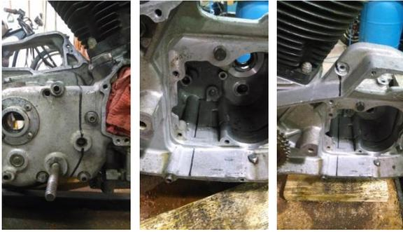
2. Rough cutting the cases. The easiest way to do this is to have the cases split, empty, and run it through a band saw. But, since most people do not have access to one we have found that a 4" cutting wheel on a hand grinder or a metal bit on a sawsall works well. If you are not intending to split the cases and rebuild you engine you will need to seal off all ports to prevent any debris from getting into the engine components. Otherwise you will be rebuilding your engine soon.
