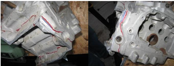
**LATE 77 & NEWER:** All excess material to be removed as shown. Bottom case bolt hole will be shortened to 5/8" for clearance of the frame. It will later be used in the installation of the rear motor mounts.
