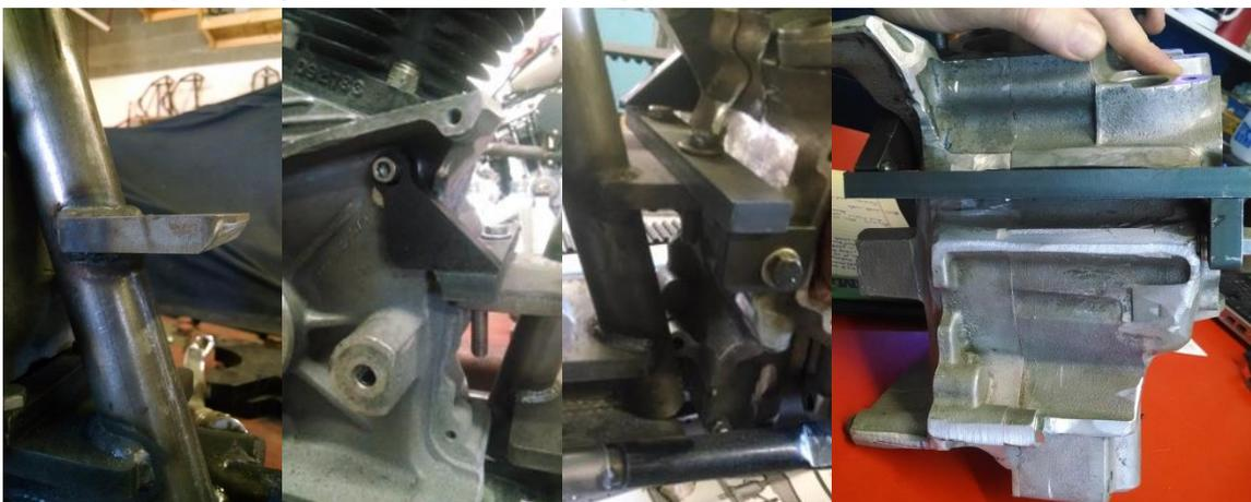
6. With the motor mounts tack welded together the engine can be removed to fully weld together. It will be a little difficult to get each location welded inside the frame.
