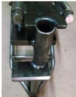
**2:** on the OEM frame half you will need to cut the frame just behind the top motor mount and replace it with a new section. The section that gets replaced will be the same diameter as the Shortsters Frame Tail Section. The change in diameter will be welded together under the gas tank and not noticed. There will also be a slight bend in the backbone when finished since the OEM frame has a slightly different angle. Once again this wont be noticed when you install a gas tank.
