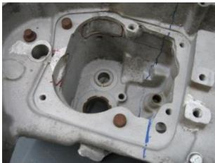
**EARLY 69 & OLDER:** you will draw and cut in the same place. You will be cutting into the oil feed line in the case. Don't worry, we will be relocating this and the vent line.
