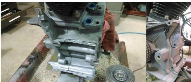
4. To remove large pieces of material use the hand grinder with the 4" cutting wheel to cut slits in the aluminum near the depth that you want. These teeth will break off easily with a flat screwdriver or a chisel. Then you can use the hand grinder with a grinding wheel to smooth out the back side and make it look nice.
