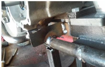
**BIG TWIN FRAMES:** With the use of both front and rear motor mounts you can install a divorced ironhead into a big twin frame. There are a few modifications to be made to the frame to get the proper fitment. **(NOTE: We have yet to do a complete build using an actual Big Twin frame. We are passing along everything that we DO know. #1 was built with a 45 Magnum frame. Its similar but not exact.)**
