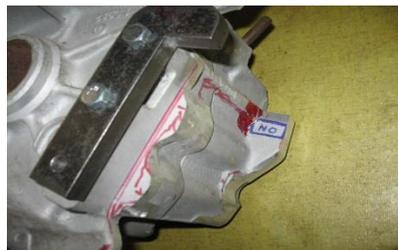
4. Fitting the top platform can be a bit tedious. You will need to make the proper clearances. This is a tight fit. Test fit the top bracket and mark the surfaces that is preventing it from lining up. You can also grind clearances in the platform itself along with the back side of the case. **DO NOT**
