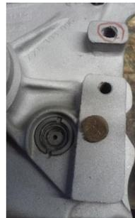
3. Attach the primary side bracket to the chain tensioner bolt holes. **DO NOT** drill the 3<sup>rd</sup> hole yet.
