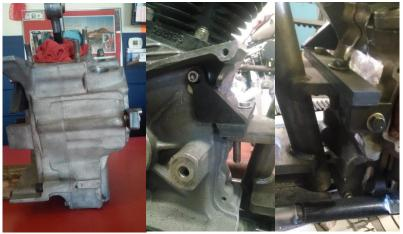
5. Fit the engine into the frame with it aligned square with the transmission. (Refer to Frames section for instructions to square up the engine) If you are using the Shortsters Frame Tail Section some material will need to be removed from the lower edge of the frame rear mount platform for it to fit the back side of the late model cases. Once the engine is square and secure in the frame you can go ahead and tack weld together.
