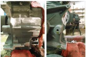
**2.** A notch needs to be cut in the casting on the primary case half as shown. This needs to be done to allow proper clearance for the primary side case bracket.
