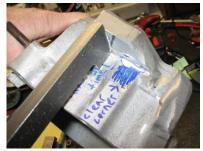
7. Remove the case bolt from behind the oil pump and file the case until the washer is proud of the casing around the faced surface of the case bolt. Once this is done the "L" bracket should fit flat to the washer **not the case.** Replace the factory case bolt with the flat head socket cap screw. Blue Loctite on final assembly.
