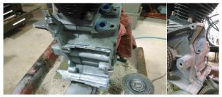
**4.** To remove large pieces of material use the hand grinder with the 4" cutting wheel to cut slits in the aluminum near the depth that you want. These teeth will break off easily with a flat screwdriver or a chisel. Then you can use the hand grinder with a grinding wheel to smooth out the back side and make it look nice.
