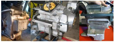
**FRONT:** The front motor mounts is NOT needed to build and original frame Shortsters conversion. The front motor mount set converts Sportster motor mounts to Big-twin style in height and longitudinal location for custom frame applications. The bar is undrilled for your desired lateral engine position.
