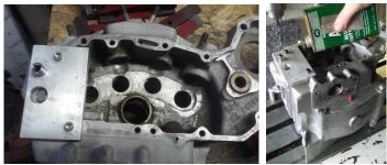
6. After the 5/16 hole is drilled through the case using the drill fixture the top platform can now be bolted in using the 15/16- 18 bolt provided. If it does not line up square then more clearance is needed somewhere. If so refer back to step #3.
