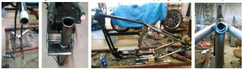
**79-81 FRAMES:** these three years of frames have an odd design. Most of this will get cut off. The only differences is the back bone. The area where it is to be plugged has been dented for factory clearance. You have two options. **1:** using a torch heat up the dented tube and pound out the dent allowing the plug to be inserted. **2:** cut out the dent and add an extention to replace the
