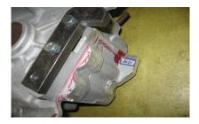
4. Fitting the top platform can be a bit tedious. You will need to make the proper clearances. This is a tight fit. Test fit the top bracket and mark the surfaces that is preventing it from lining up. You can also grind clearences is the platform itself along with the back side of the case. **DO NOT**
