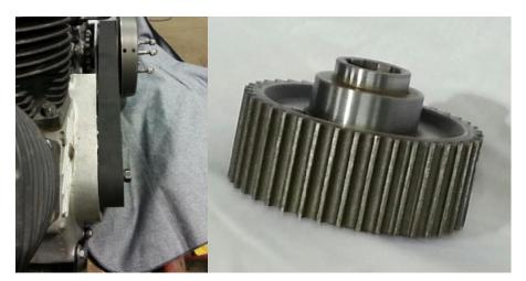
The belt drive is a modified Karata and the 8.07 mm belt will **NOT** exchange with any other belt or pulleys. The ratio is for Shovelhead but our Shortsters lose 100 lbs and you have the option of the bagger 1<sup>st</sup> gear and unlimited adjustment of overall gearing at wheel or transmission sprocket.
