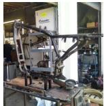
**1:**On the Shortsters Frame Tail Section you will need to remove some material from the edge of the plate that sits in between the bottom frame rails to acomidate the larger diameter of the OEM frame half.
