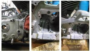
2. Rough cutting the cases. The easest way to do this is to have the cases split, empty, and run it through a band saw. But, since most people do not have access to one we have found that a 4" cutting wheel on a hand grinder or a metal bit on a sawsall works well. If you are not intending to split the cases and rebuild you engine you will need to seal off all ports to prevent any debris from getting into the engine components. Otherwise you will be rebuilding your engine soon.
