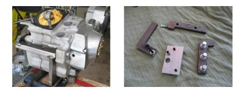
NEEDED TOOLS: Drill, 5/16 drill bit, 3/8-16 tap, rotary file/grinder, allen wrenches, blue Loctite, welder
