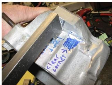
7. Remove the case bolt from behind the oil pump and file the case until the washer is proud of the casing around the faced surface of the case bolt. Once this is done the "L" bracket should fit flat to the washer **not the case**. Replace the factory case bolt with the flat head socket cap screw. Blue Loctite on final assembly.
