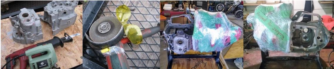
3. I now pronounce you divorced!.....roughly. With the transmission case divorced from the engine you can see all the excess material that needs to be removed. Using the permanent marker identify all the excess material you will need to be removing.
