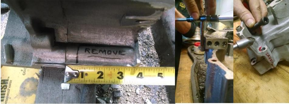
4. On both sides of the cases remove the proper case bolts. Using the supplied hardware attach both side brackets with the proper washers to space out the brackets so they clear the cases. The side brackets rest on the washers, **NOT** the cases. Usually no more than 2/side is needed.
