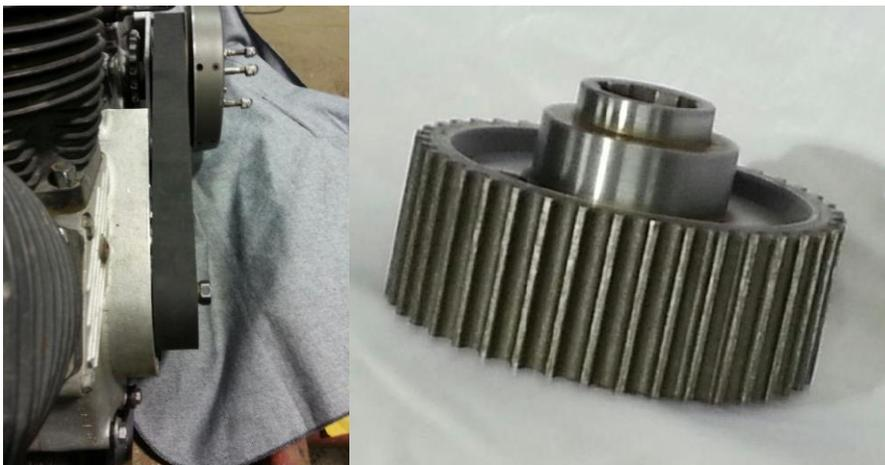
The belt drive is a modified Karata and the 8.07 mm belt will **NOT** exchange with any other belt or pulleys. The ratio is for Shovelhead but our Shortsters lose 100 lbs and you have the option of the bagger 1<sup>st</sup> gear and unlimited adjustment of overall gearing at wheel or transmission sprocket.
