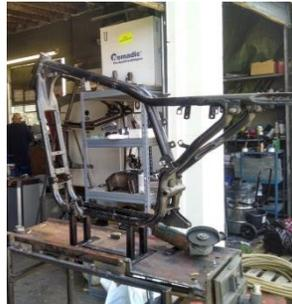
**1:**On the Shortsters Frame Tail Section you will need to remove some material from the edge of the plate that sits in between the bottom frame rails to acomidate the larger diameter of the OEM frame half.
