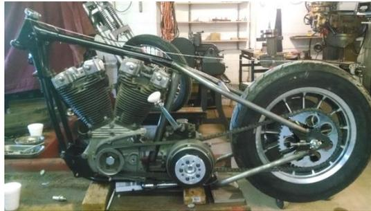
4. Once you have everything plugged, aligned, and square weld the frame halves together. Now is also the time when you can go ahead and weld the motor mount brackets together.
