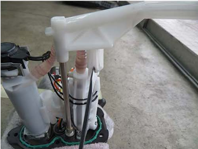
15, When the vent tube is loosened about half way, release the lock tab on the top plastic part with a flat head screw driver.
