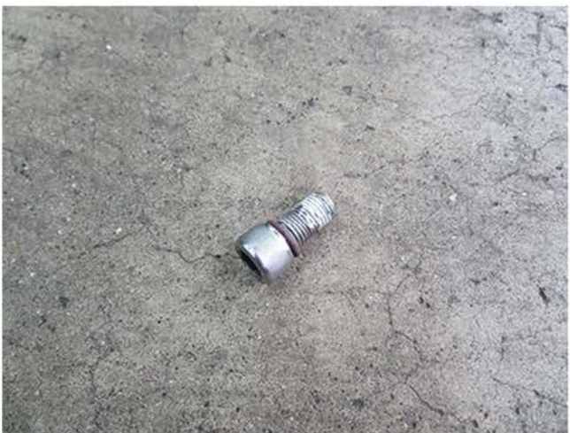
17, Install the O-ring onto the 3/8" Allen head bolt that come in this kit. *Apply some sealant onto the bolt thread in order to prevent gasoline leakage.
