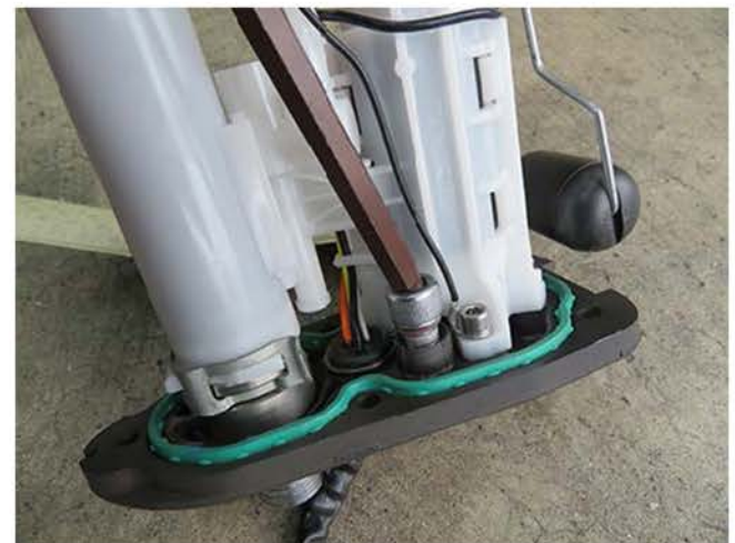
18, Install the Allen head bolt into the screw hole where the vent tube was originally located.
