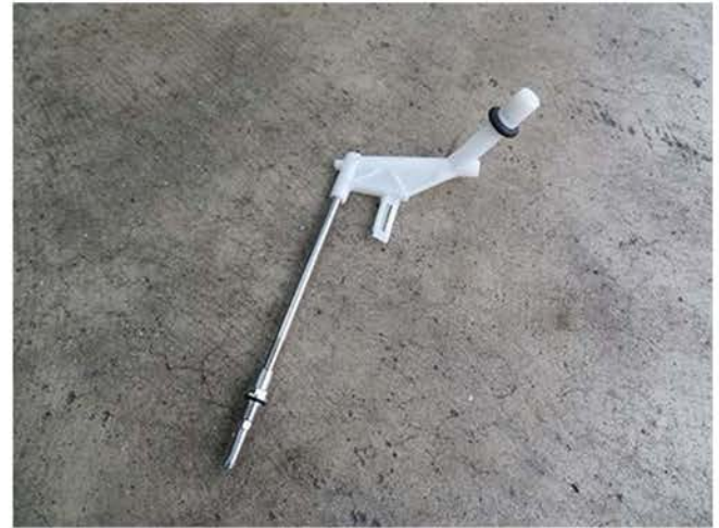
16, Loosen the vent tube all the way to remove off the assembly. *This part will not be re-used with the new fuel tank.
