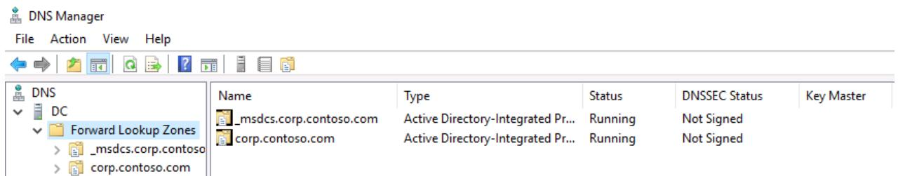
The screenshot shows the Windows DNS Manager application. The left pane displays a tree view of DNS zones under 'DC' (Domain Controller), specifically 'Forward Lookup Zones'. The right pane is a grid table with columns: Name, Type, Status, DNSSEC Status, and Key Master. It lists two zones: '\_msdcs.corp.contoso.com' and 'corp.contoso.com', both of which are 'Active Directory-Integrated Pr...' and 'Running'. The 'DNSSEC Status' column indicates 'Not Signed' for both entries.
