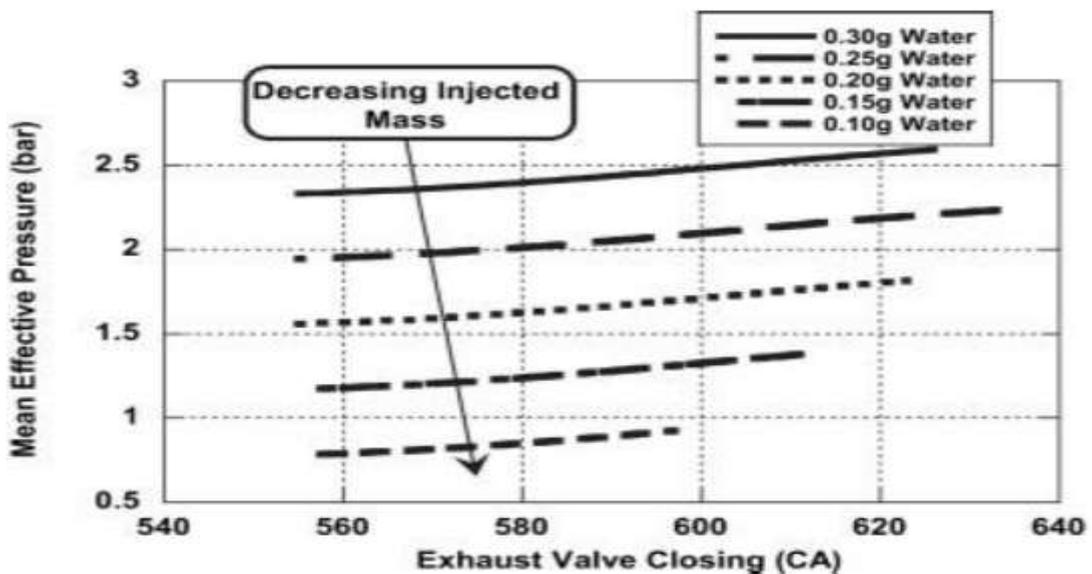
Mean effective pressure due to second expansion with water injection in HP cylinder
