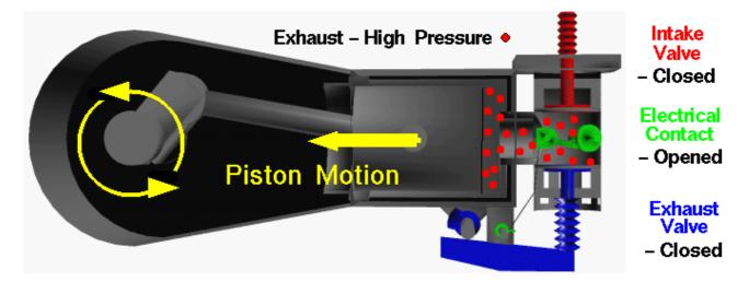
Unlike the compression stroke, the hot gas does work on the piston during the power stroke. The force on the piston is transmitted by the piston rod to the crankshaft, where the linear motion of the piston is converted to angular motion of the crankshaft. The work done on the piston is then used to turn the shaft, and the propellers, and to compress the gases in the neighboring cylinder's compression stroke. Having produced the igniting spark, the electrical contact remains opened.
