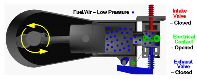
The cylinder and combustion chamber are full of the low pressure fuel/air mixture and, as the piston begins to move to the right, the intake valve closes.
