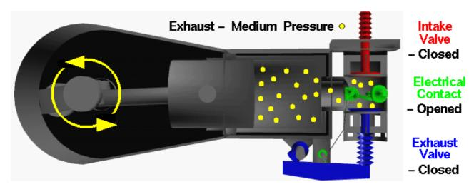
**Historical note -** The method of producing the electrical spark used by the Wright brothers is called a "make and break" connection. There are moving parts located inside the combustion chamber. Modern internal combustion engines do not use this method, but instead use a spark plug to produce the ignition spark. A spark plug has no moving parts, which is much safer than the method used by the brothers.
