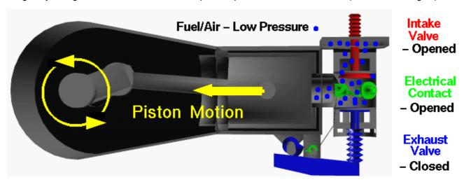
The intake valve is open, and fuel and air are drawn past the valve and into the combustion chamber and cylinder from the intake manifold located on top of the combustion chamber. The exhaust valve is closed and the electrical contact switch is open. The fuel/air mixture is at a relatively low <u>pressure</u> (near atmospheric) and is colored blue in this figure. At the end of the intake stroke, the piston is located at the far left and begins to move back towards the right.
