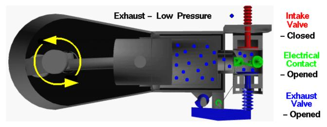
The purpose of the exhaust stroke is to clear the cylinder of the spent exhaust in preparation for another ignition cycle. As the exhaust stroke begins, the cylinder and combustion chamber are full of exhaust products at low pressure (colored blue on the figure above.) Because the exhaust valve is open, the exhaust gas is pushed past the valve and exits the engine. The intake valve is closed and the electrical contact is open during this movement of the piston.
