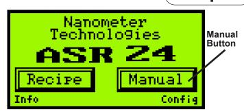
1) Press the Manual Button on the touchscreen to open the Manual Mode Recipe screen.
