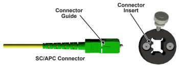
Insert the SC/APC Connectors into the Fixture Plate. Note that the guide on the top of the connector slides into a slot located in the Connector Insert of the Fixture Plate. Make sure the connector has been pushed to the bottom of the Connector Insert.
