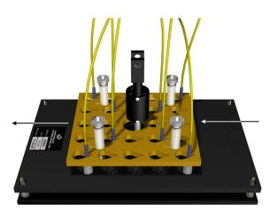
**3)** Loosen the **Locking Plate** and slide it over the connectors, then re-tighten the **Locking Plate**. Tighten nuts diagonally.
