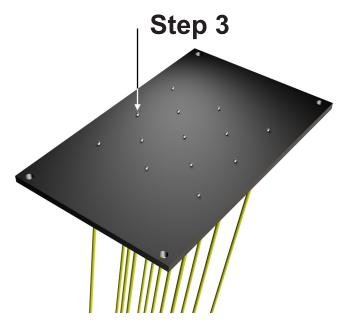
**3)** Lift up plate and press on the ferrules, checking to make sure the connectors have spring action and none are locked in place. Place the **Fixture Plate** back onto the **Fixture Holder**.
