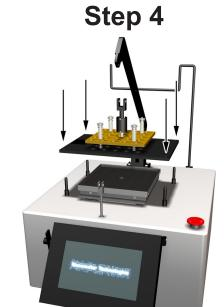
**4)** Place the **Fixture Plate** on the ACP 24. Make sure the **Fixture Plate** fits onto the 4 locator pins.
