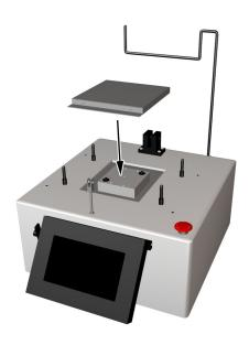
**3)** Set the **Base Plate** on the **Interface Plate**. Make sure both surfaces are clean. Use the guide holes on the **Base Plate** to line up with the **Interface Plate**.
