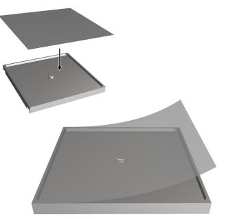
**2)** Set the ASR Fixture Plate with the raised center face up. Place the **15 micron silicon carbide film** (with PSA backing) onto the **ASR Plate**. Start on an edge and slowly roll across the fixture plate.
