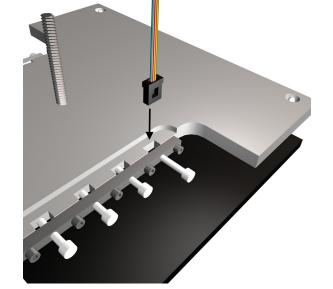
**3)** Loosen the **Nylon Screws** that will hold the connectors.
