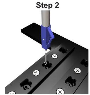
**2)** Place the **LC connector** into a connector slot with the locking arm facing the notched side of the connector slot as shown. if done properely the connector will snap into place.
