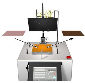
**9a)** Replace the **6um Diamond Film** with the **3um Diamond Film**.
