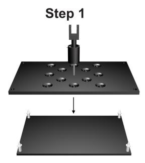
1) Make sure the Fixture Plate is free of particles.
