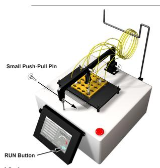
**10c)** Lower the polishing plate onto the 4 locating pins making sure that it lies flat on the base plate.
