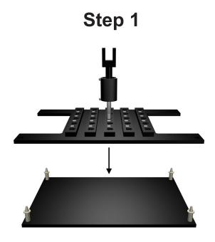
1) Place the Polishing Fixture on the Fixture Holder.
