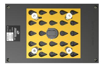
**2)** Loosen the nuts that hold down Locking Plate and slide it until the large end of the tear drop holes line up with the holes on the **Polishing Fixture**.
