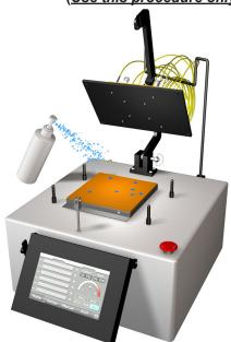
**7a)** Apply a very small amount of distilled water to the rubber surface using the spray bottle.
