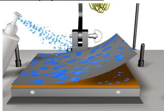
**7b)** Place the **15 um silicon carbide film** with the smooth shiny side down on the **Rubber Pad**.
