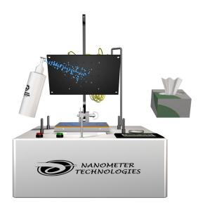
**10d)** After polishing has finished, remove the small pushpull pin and lift the polishing plate.
