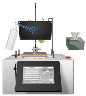
**9d)** After polishing has finished, remove the small pushpull pin and lift the polishing plate.
