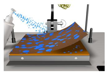
**8b)** Place the **6 um Diamond film** with the smooth shiny side down on the rubber pad.
