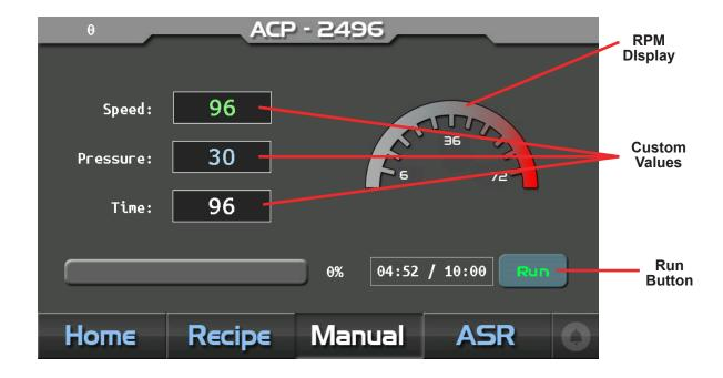
The Manual Screen is for running a quick custom polishing step.
