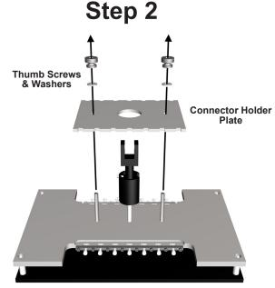
2) Remove the **Thumb Screws & Washers**. Lift and remove the .
