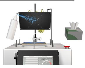
**7d)** After polishing has finished, remove the small push-pull pin and lift the polishing plate.
