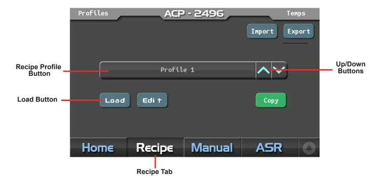
1) Press the **Recipe Tab** on the bottom of the screen. Press the **Profile Button** to select a **Fixture Plate**. Use the **Up/ Down Arrows** to find the fixture plate. With the fixture plate selected, press the **Load Button**. Return to the home page by pressing the **Home Tab**.
