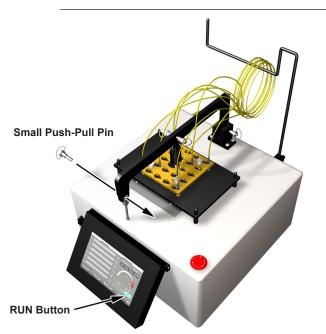
**9c)** Lower the polishing plate onto the 4 locating pins making sure that it lies flat on the base plate.
