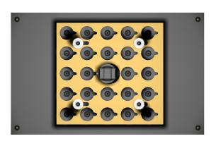
**2)** Loosen the nuts that hold down Locking Plate and slide it until the large round holes are centered with the holes on the Polishing Fixture.
