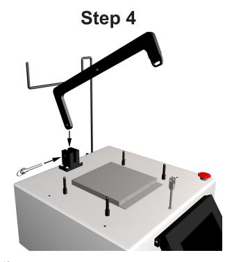
4) Take the Pneumatic Arm and place the longer end into the Delrin Bracket located in the rear-center of the polisher. Line up the open holes. Take the Large Push-Pull Locking Pin and push in and hold the Lock-Release Button located on the end of the pin. Insert the pin into the hole and release the Lock-Release Button.
