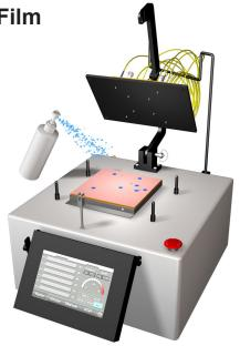
**9b)** Spray distilled water onto the surface of the film and wipe clean using lint-free wipes. This procedure will ensure a clean working surface and remove any large air bubbles.
