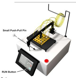
**8c)** Lower the polishing plate onto the 4 locating pins making sure that it lies flat on the base plate.
