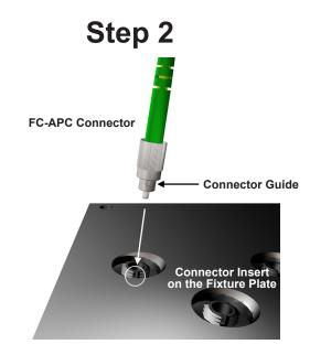
**2)** Insert the FC/APC Connectors into the Fixture Plate. Make sure the guide on the Connector is aligned with the slot on the Fixture Plate.
