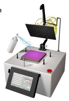
**10b)** Spray distilled water onto the surface of the film and wipe clean using lint-free wipes. This procedure will ensure a clean working surface and remove any large air bubbles.
