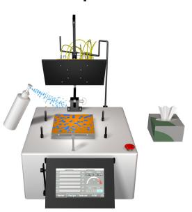
**6)** Lift the arm to expose the **Rubber Pad**. Spray distilled water onto the Rubber Pad and use a **Lint-Free Optical Wipe** to clean the surface.
