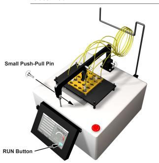
**7c)** Lower the polishing plate onto the 4 locating pins making sure that it lies flat on the base plate.
