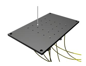
**4)** Lift up plate and press on the ferrules, checking to make sure the connectors have spring action and none are locked in place. Place the **Fixture Plate** back onto the **Fixture Holder**.
