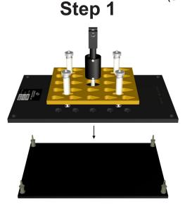
1) Make sure the **Fixture Plate** is free of particles. Place the **Polishing Fixture** on the **Fixture Holder**.
