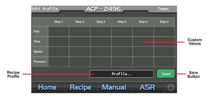
Use the Edit Recipe function to create custom polishing recipes or make adjustments to existing recipes. Press an empty box under each step to enter a custom configuration.
