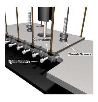
**4b)** Tighten the **Thumb Screws** first. Then tighten the **Nylon Screws** to hold the ferrules in place.
