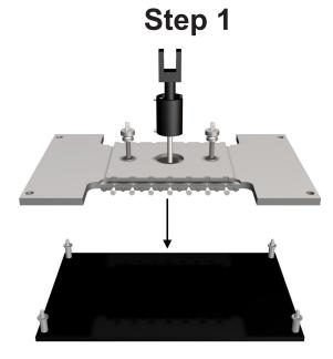
1) Place the Fixture Plate on the Fixture Holder.
