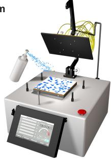
**11b)** Spray distilled water onto the surface of the film and wipe clean using lint-free wipes. This procedure will ensure a clean working surface and remove any large air bubbles.
