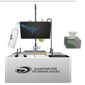
**8d)** After polishing has finished, remove the small pushpull pin and lift the polishing plate.
