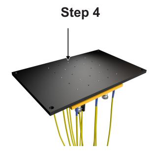
**4)** Lift up plate and press on the ferrules, checking to make sure the connectors have spring action and none are locked in place. Place the **Fixture Plate** back onto the **Fixture Holder**.
