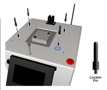
**2)** Insert the **Fixture Plate Locator Pins.** The inner holes are for MCP 24 Fixture Plates. The outer holes are for MCP 48 Fixture Plates.
