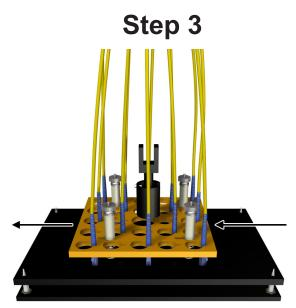
**3)** Loosen the **Locking Plate** and slide it over the connectors. Then retighten the **Locking Plate**. Tighten nuts diagonally.
