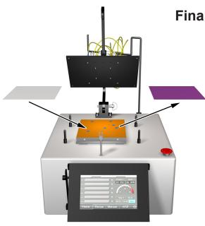
**11a)** Replace the **1 um Diamond Film** with the **Final Polishing Film**.
