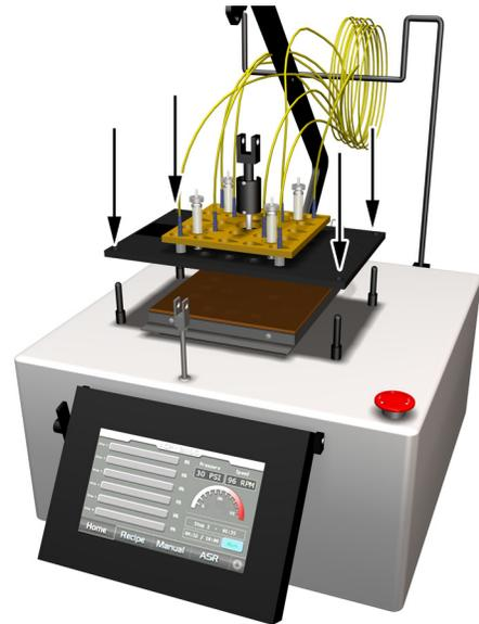
4) Place the fiber optic cables onto the Cable Tree.
