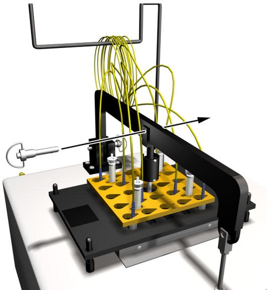
5) Lower the **Pneumatic Arm** onto the **Polishing Fixture Bracket**. Use the **Medium Push-Pull Locking Pin** to attach the **Polishing Fixture** to the **Pneumatic Arm**.
