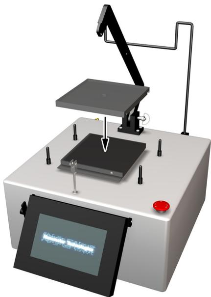
3) Place the **ASR Fixture Plate** onto the **Base Plate**.
