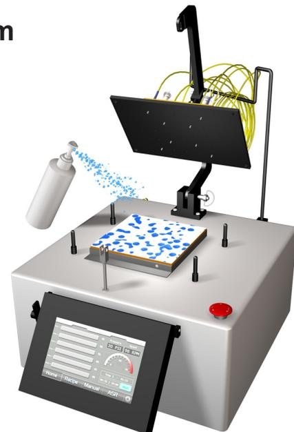
**11b)** Spray distilled water onto the surface of the film and wipe clean using lint-free wipes. This procedure will ensure a clean working surface and remove any large air bubbles.
