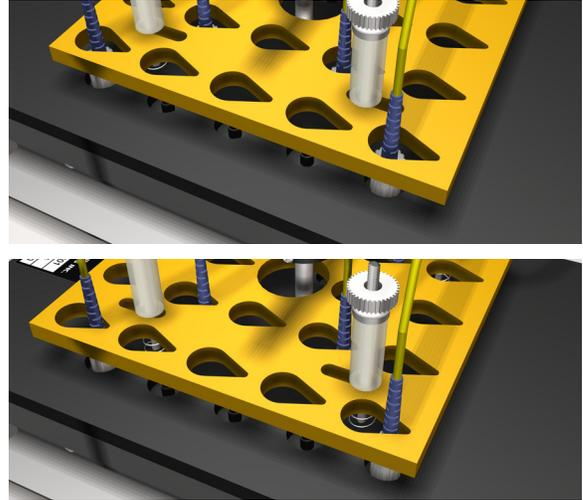
6) Carefully lift the **Slider Plate** and gently place over the top of connectors. Make sure the small end of the tear drop is touching the **Connector Boots**.
