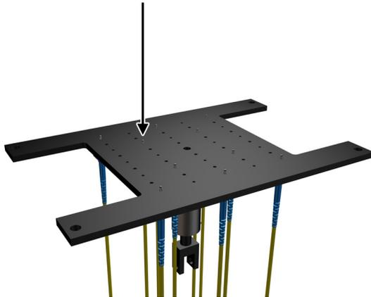
**3)** Lift up plate and carefully press on the ferrules, checking to make sure the connectors have spring action and none are locked in place. Pressing too hard may cause a connector to pop free. Place the Fixture Plate back onto the Fixture Holder.
