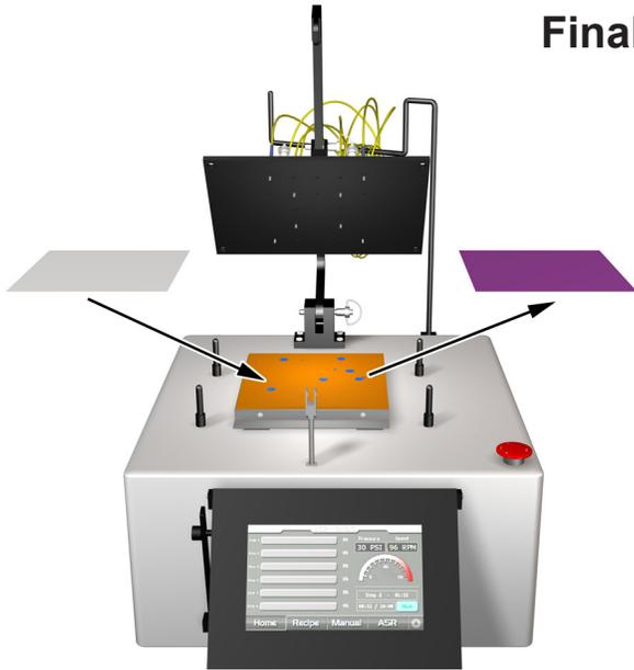
**11a)** Replace the 1 um Diamond Film with the Final Polishing Film.
