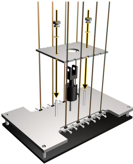
**4a)** Re-install the **Connector Holding Plate**, **Thumb Screws**, and **Washers**.
