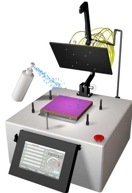
**10b)** Spray distilled water onto the surface of the film and wipe clean using lint-free wipes. This procedure will ensure a clean working surface and remove any large air bubbles.
