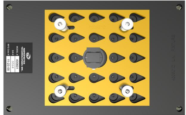
**2)** Loosen the nuts that hold down **Locking Plate** and slide it until the large end of the tear drop holes line up with the holes on the **Polishing Fixture**.
