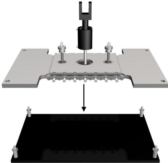
1) Place the **Fixture Plate** on the **Fixture Holder**.
