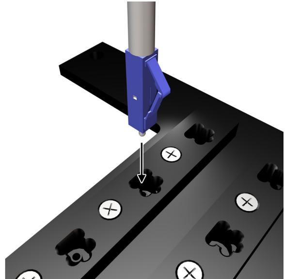
**2)** Place the **LC connector** into a connector slot with the locking arm facing the notched side of the connector slot as shown. If done properly the connector will snap into place.
