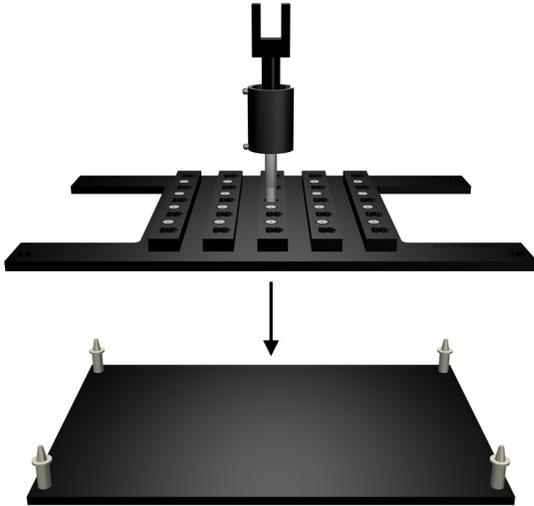
**1)** Place the **Polishing Fixture** on the **Fixture Holder**.
