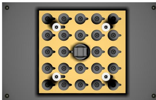
**2) Loosen the nuts that hold down Locking Plate and slide it until the large round holes are centered with the holes on the Polishing Fixture.**
