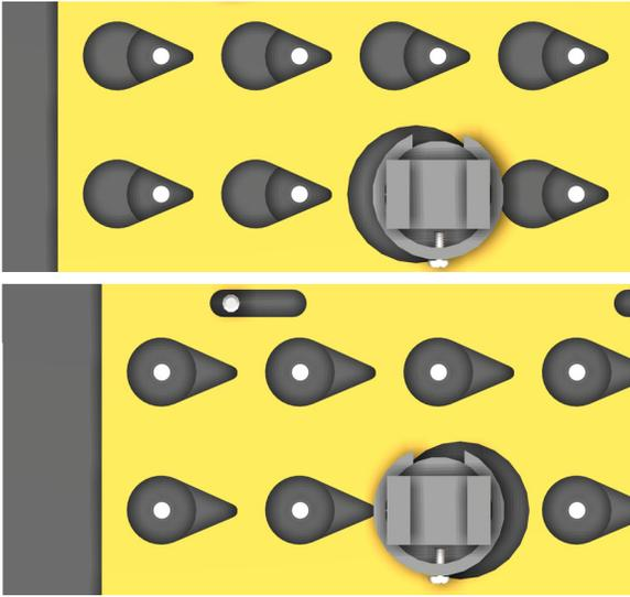
5) Adjust the **Slider Plate** until the connector slot lines up with the bottom edge of the tear drop shape. This will make it easier to load the connectors.
