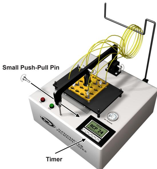
**11c)** Lower the polishing plate onto the 4 locating pins making sure that it lies flat on the base plate.
