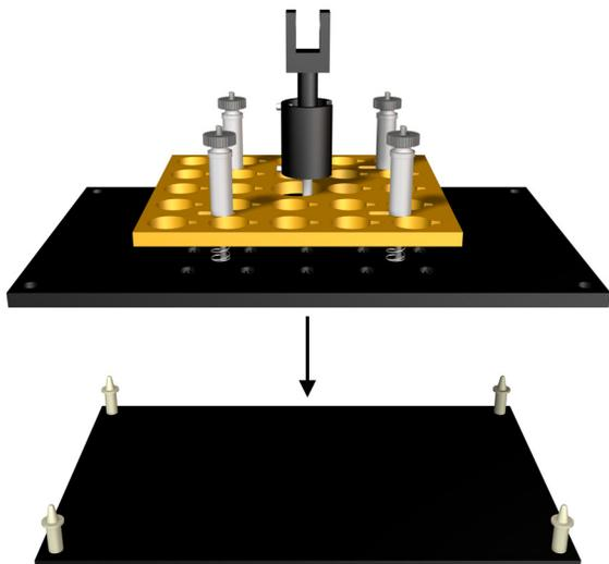
**1) Place the Polishing Fixture on the Fixture Holder.**
