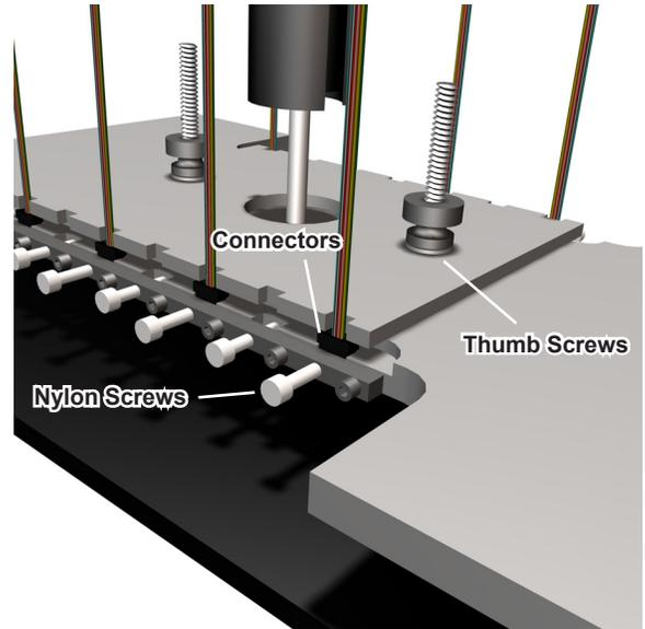
**4b)** Tighten the **Thumb Screws** first. Then tighten the **Nylon Screws** to hold the ferrules in place.
