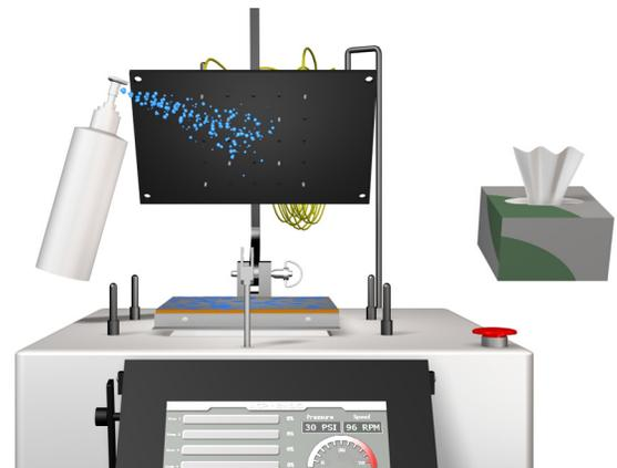
**7d)** After polishing has finished, remove the small push-pull pin and lift the polishing plate.
