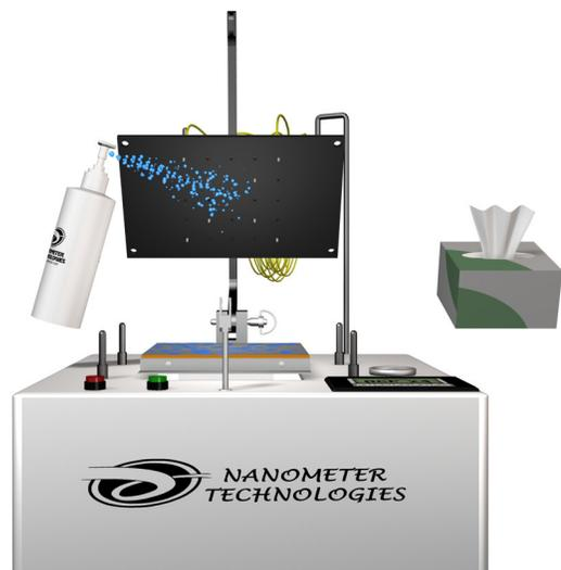
**10d)** After polishing has finished, remove the small push-pull pin and lift the polishing plate.
