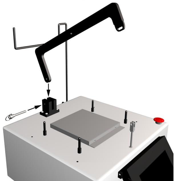
**4)** Take the **Pneumatic Arm** and place the longer end into the **Delrin Bracket** located in the rear-center of the polisher. Line up the open holes. Take the **Large Push-Pull Locking Pin** and push in and hold the **Lock-Release Button** located on the end of the pin. Insert the pin into the hole and release the **Lock-Release Button**.
