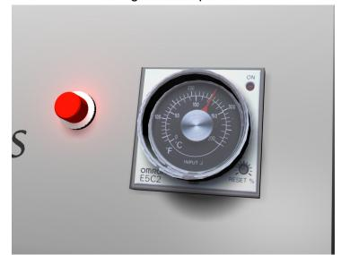
Set the **Oven** temperature to the epoxy manufacturer's temperature recommendation. Turn the dial to the desired temperature level.
